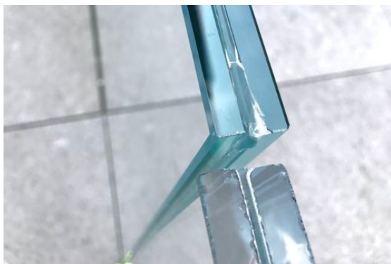
Fig. 8. Oldcastle low-iron glass, showing center PVB lamination.
