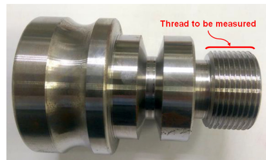
Fig. 1 Workpiece sample and tread to be measured in this study.
