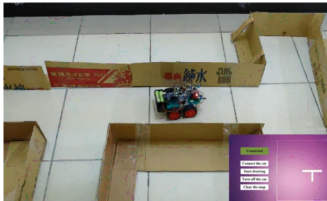
Fig. 9. User interface and actual automatic path drawing car driving.
