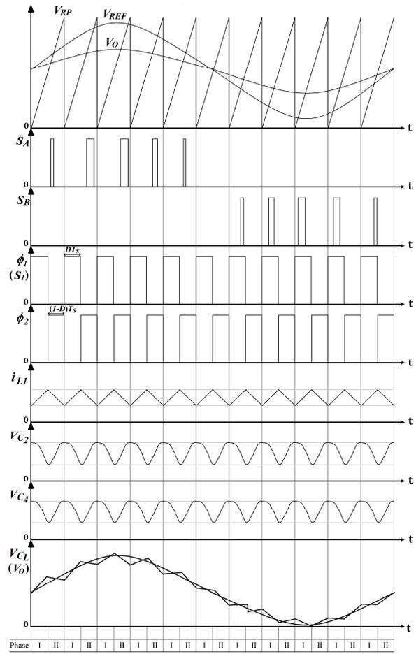
Fig. 2. Theoretical waveforms of CICWSC.
