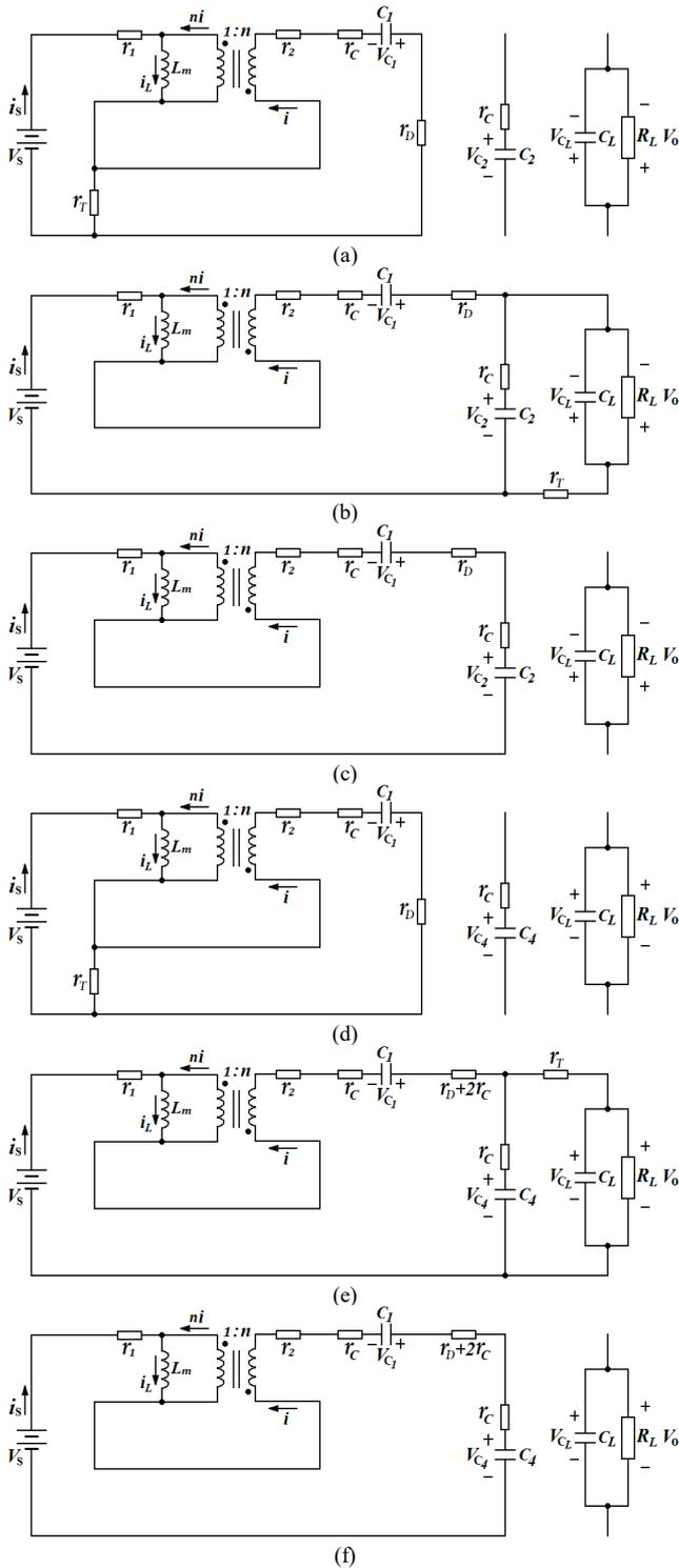
Fig. 4. Effective circuits heading for negative output in Phase (a) I, (b) II while  $S_B$ : SPWM-ON, (c) II while  $S_B$ : SPWM-OFF; Effective circuits heading for positive output in Phase (d) I, (e) II while  $S_A$ : SPWM-ON, (f) II while  $S_A$ : SPWM-OFF.
