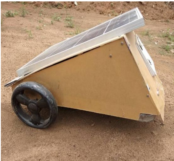
Fig 7: Side view of the constructed Automated Lawn Mower
