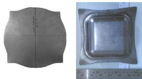
Fig. 15: (a) Optimum blank; (b) Drawn optimum blank.
