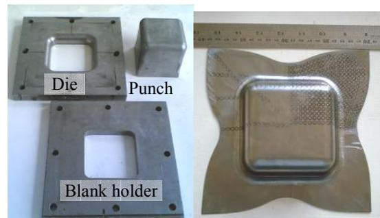
Fig. 14: (a) Die set components; (b) Drawn blank.
