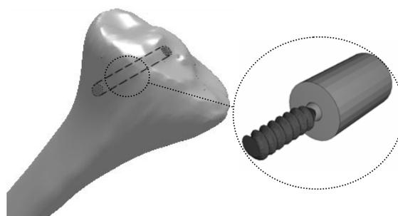
Fig. 3. Schematic of a tibia bone with a cylindrical tunnel. The model assumes a cylindrical section of bone around the tibia tunnel.
