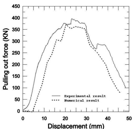
Fig. 2. Pulling force versus displacement of a porcine bone and calf tendon fixed at one end.
