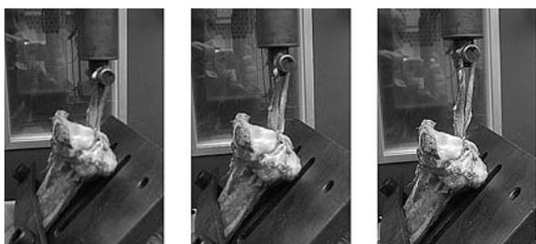
Fig. 1. Mechanical testing of porcine/calf tibial bone and tendon graft (tunnel is 45 degree from central axes of the bone). The pulling force and axis of the tunnel are in the same direction.
