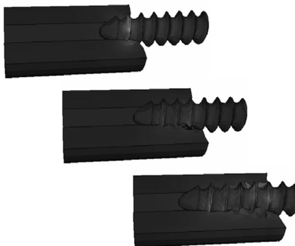
Fig. 4. Von Mises stresses in the tibia finite element model of the region around the screw (the screw was inserted into tunnel by combined axial/rotational movement).
