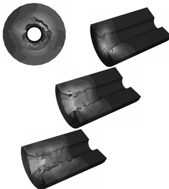
Fig. 5. Von Mises stress contour plots of transverse sections of tibia.
