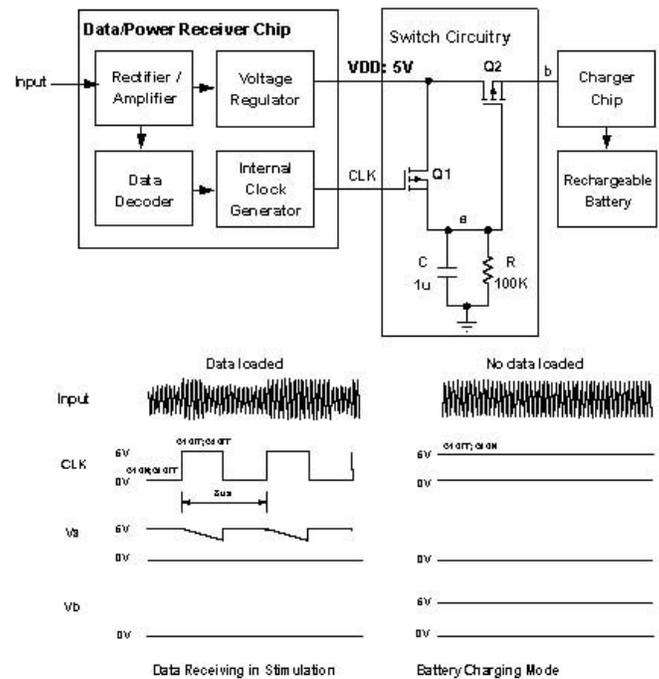
Fig. 2 Operation of switch circuitry in stimulation and battery charging modes
