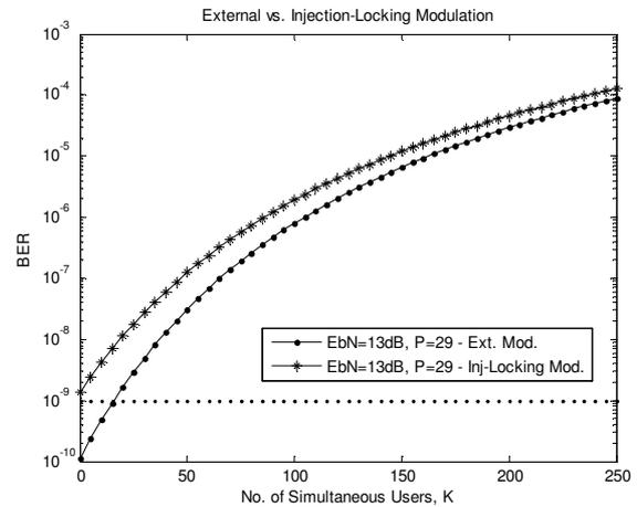
Fig. 5. Performance comparisons of externally and injection-locking modulated BPSK-OCDMA system versus number of simultaneous active users ( $K$ )
