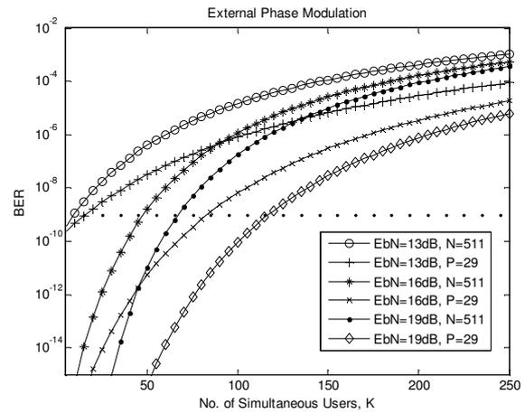
Fig. 4. Performance of BPSK-OCDMA system using an external modulator versus number of simultaneous active users ( $K$ )
