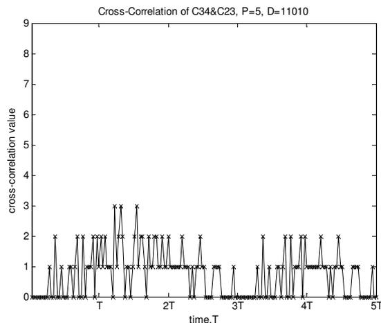
Fig. 3. Cross-correlation values of  $C_{34}$  and  $C_{23}$  (Different Groups) DPMP for data stream '11010'. ( $T$  is synchronization time)
