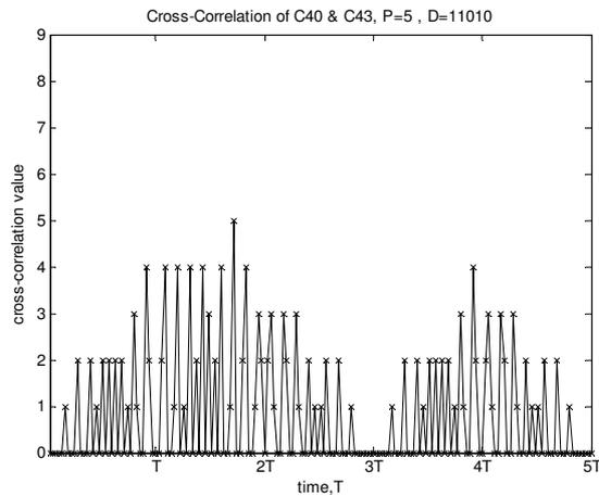
Fig. 2. Cross-correlation values of  $C_{40}$  and  $C_{43}$  (Same Group) DPMP for data stream of '11010'. ( $T$  is synchronization time)
