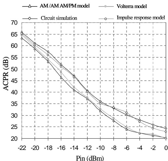
Fig. 6. ACPR=f(Pin) 16-QAM @ 5 Mbits/s.
