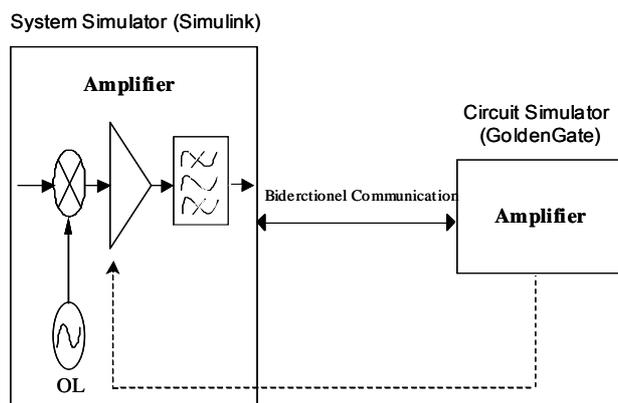
Fig. 5. Co-simulation principle
