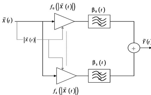
Fig. 2. Nonlinear impulse response model
