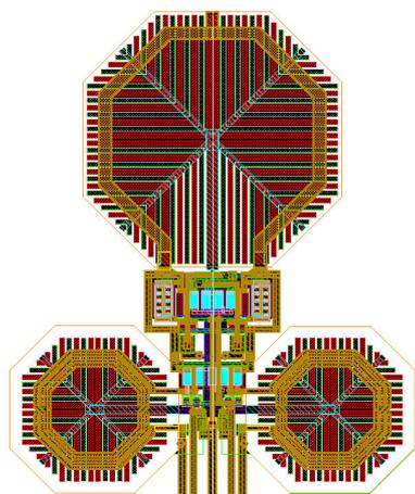
Fig. 9 20 GHz SiGe:C LC-VCO cross-coupled differential pair layout measuring 305  $\mu\text{m}$  x 405  $\mu\text{m}$
