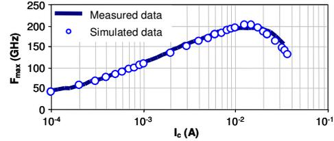
Fig. 4 Cut-off frequency  $f_{max}$ -versus collector current  $I_C$
