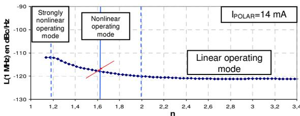
Fig. 7 Phase noise at 1 MHz (dBc/Hz) from the carrier versus capacitances ratio  $n$  (bias current  $I_{polar} = 14$  mA)
