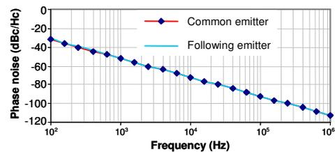
Fig. 8 Phase noise due to noise sources of cross-coupled transistors for the two buffers configurations
