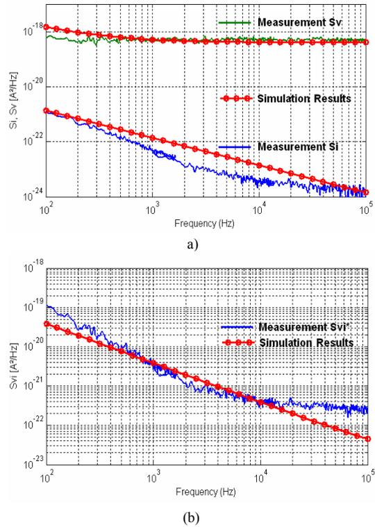
Fig. 5 (a)  $S_V$  and  $S_I$  spectra and (b) their cross-spectrum  $S_{VI}^*$ , simulated and measured. The spectra obtained with the HBT, respectively, biased at  $I_B=1 \mu A$ ,  $I_C=1.3 \text{ mA}$ . The HBT under test features an emitter area of  $0.17 \mu m \times 6.2 \mu m$
