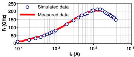
Fig. 3 Cut-off frequency  $f_T$  versus collector current  $I_C$
