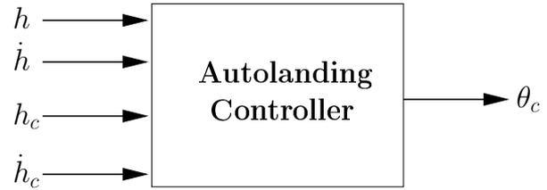
Figure 1: The controller structure for the autoland problem.
