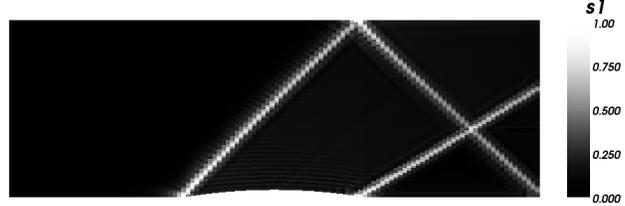
Figure 12  $s_1$  contours for circular arc test case, 120x80
