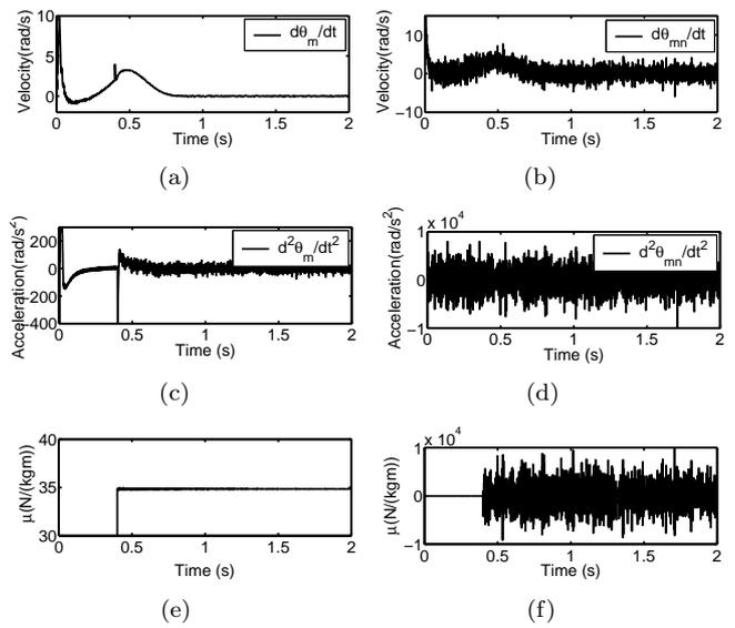
Figure 7: (a) Algebraic Estimation of  $\dot{\theta}_m$ . Numerical estimation of the motor velocity  $\dot{\theta}_{mn}$ . (c) Algebraic Estimation of  $\ddot{\theta}_m$ . (d) Numerical Estimation of the motor acceleration  $\ddot{\theta}_{mn}$ . (e) Estimation of  $\mu$  with algebraic estimates of the states. (f) Estimation of  $\mu$  with numerical estimates of the states.
