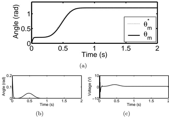
Figure 5: (a) Trajectory tracking.(b) Trajectory tracking error. (c) Control input voltage to the dc motor.
