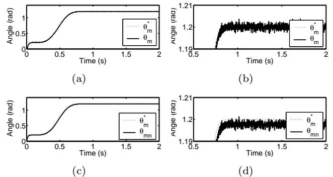
Figure 8: (a) Trajectory tracking with algebraic PD adaptive control. (b) Zoom of the trajectory tracking with algebraic PD adaptive control. (c) Trajectory tracking with adaptive PD control with numerical estimates  $\dot{\theta}_{mn}$ . (d) Zoom of the trajectory tracking with adaptive PD control with numerical estimates  $\dot{\theta}_{mn}$ .
