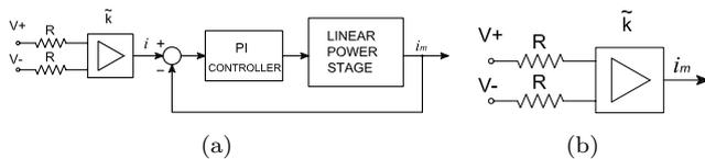
Figure 1: (a) Complete amplifier scheme.(b) Equivalent amplifier scheme.
