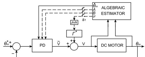
Figure 2: closed loop adaptive system
