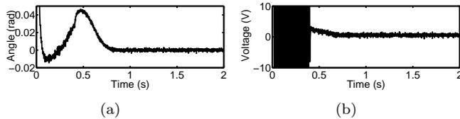
Figure 9: (a) Trajectory tracking error with algebraic PD adaptive control. (b) Control input voltage of the algebraic PD adaptive control.
