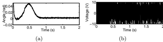
Figure 10: (a) Trajectory tracking error with PD control with numerical estimates  $\hat{\theta}_{mn}$  and  $\hat{\ddot{\theta}}_{mn}$ . (b) Control input voltage of the PD controller with numerical estimates of the states.
