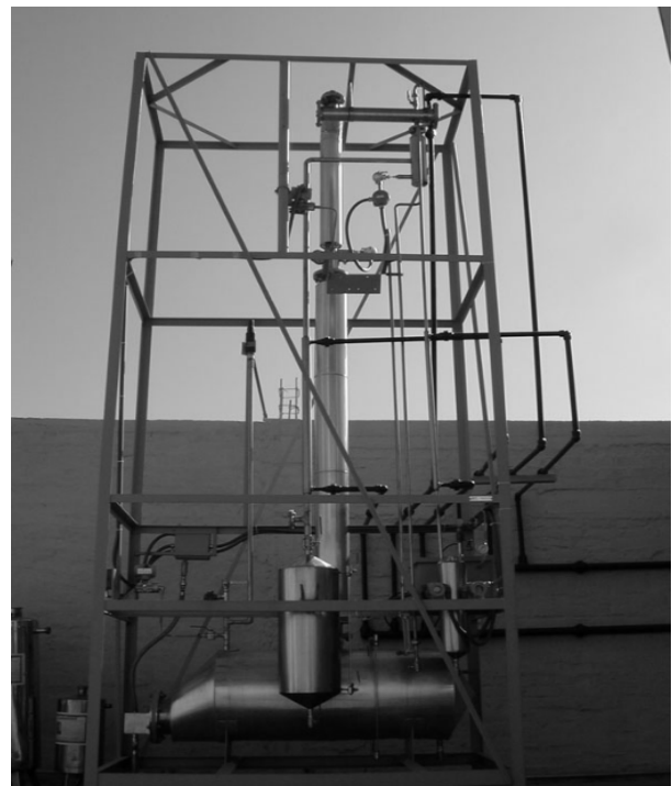
Figure 2. Discontinuous distillation plant
