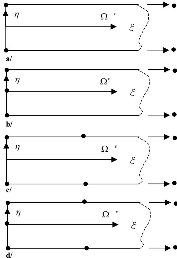
Fig.2 Infinite element domains
