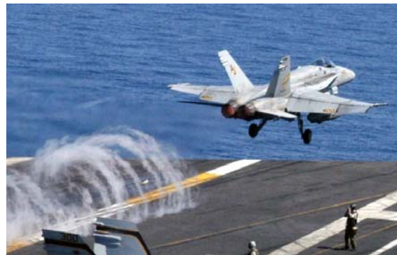
Fig. 1 Wake vortex in the take-off phase
