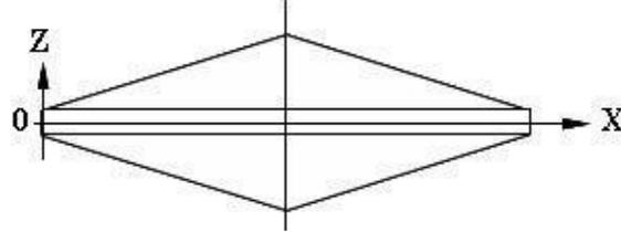
Figure 4. Plan view of a constant stress beam of variable width modified for ease of mounting
