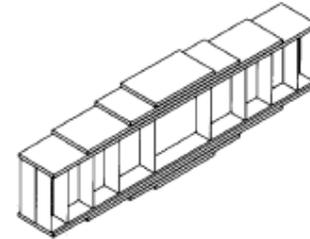
Figure 6. An I-Beam with variable flange thickness and high mass efficiency
