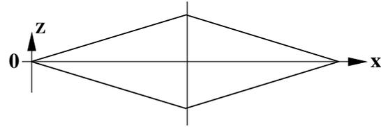
Figure 3. Plan view of a 'constant stress' beam of variable width
