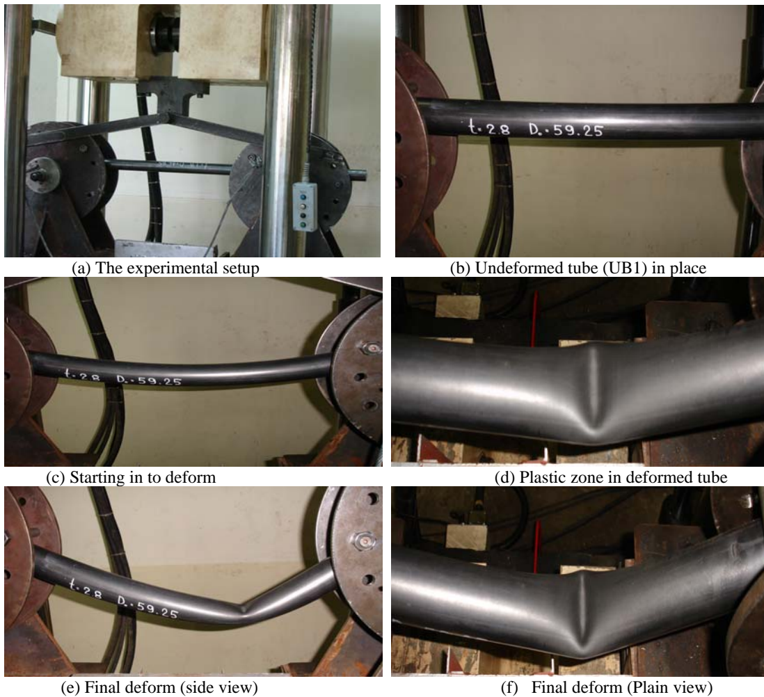
Fig. 3 The experimental setup, undeformed and deformed specimen in various views
