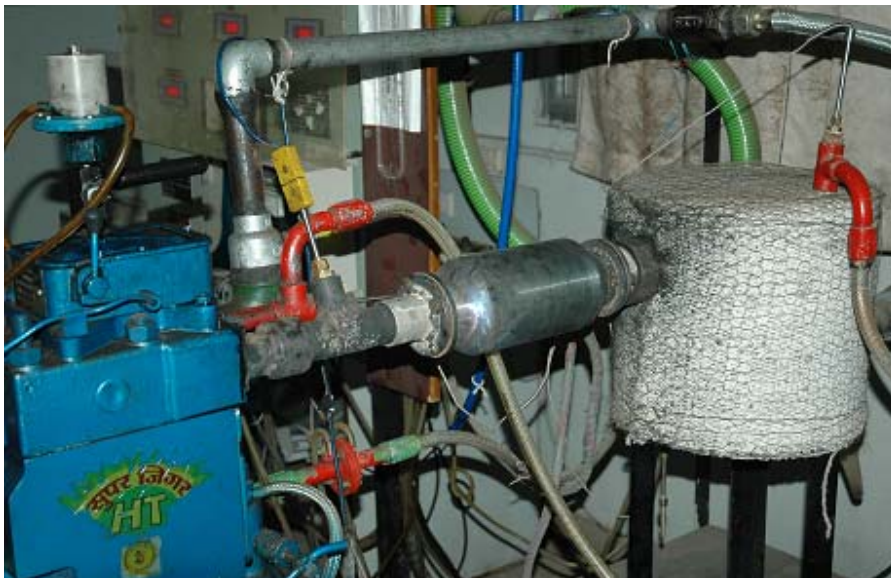
Figure IX : Diesel engine set up with Catalytic converter.
