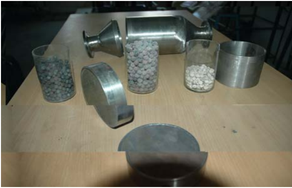
Figure VII: Catalytic converter, catalysts coated pellets and circular housing.
