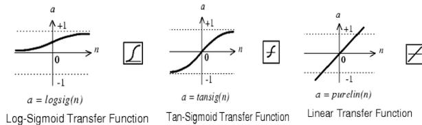
Fig. 2. Types of transfer functions.
