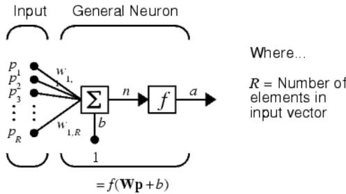
Fig. 1. Illustration of an elementary neuron.
