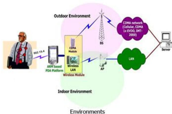
Figure 6. Communication environment of implemented system.
