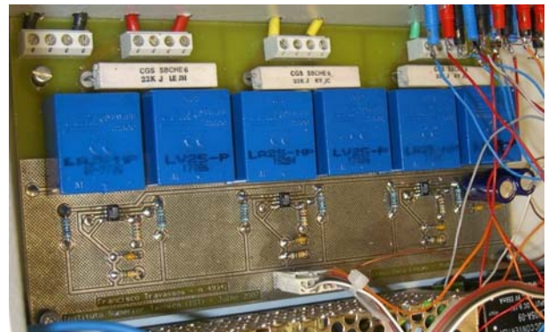
Fig. 8 – Photograph of the three-phase power measurement board.
