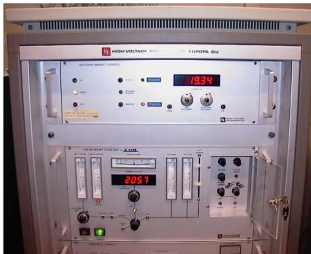
Fig. 3 – Particle accelerator control console.
