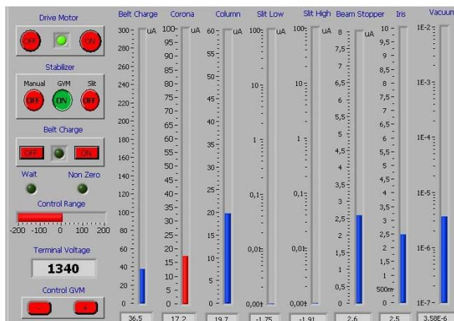
Fig. 15 – Illustration of the indicators available for the user to monitor the status of the particle accelerator.
