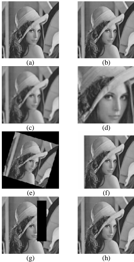
Fig. 1. (a) Original Lena Image; (b) Watermarked Lena Image; (c)-(h) Results of watermarked images with some attacks: (c) Low Pass Filtered (d) Scaled (e) Rotated (17°) (f) Cropped from top and left border (g) random modification (h) JPEG lossy compression (quality factor = 90).
