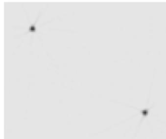
Fig. 2. Reconstructed image (zoom x3) for two 68-Ge line sources (40 cm apart) used to determine the pixel size as well as the transaxial resolution.
