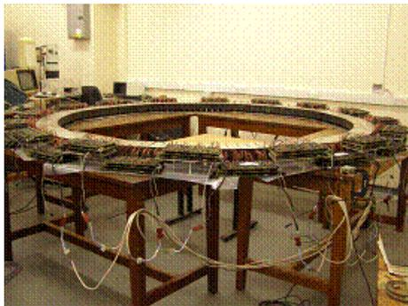
Fig. 1. Photograph of the macroPET scanner.
