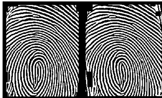
Figure 1. The left binary image is the one without the mass-centroid-based alignment. The right binary image is rotated based on the mass-centroid concept.
