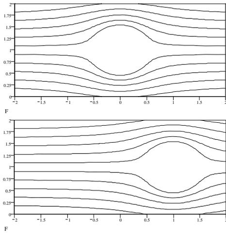
In the following figure there are represented the numerical results obtained for different position of two circular obstacles situated between the walls. Both have the same radius, and their centers are situated at the same distances from the walls, but different distances between their centers have been considered.
