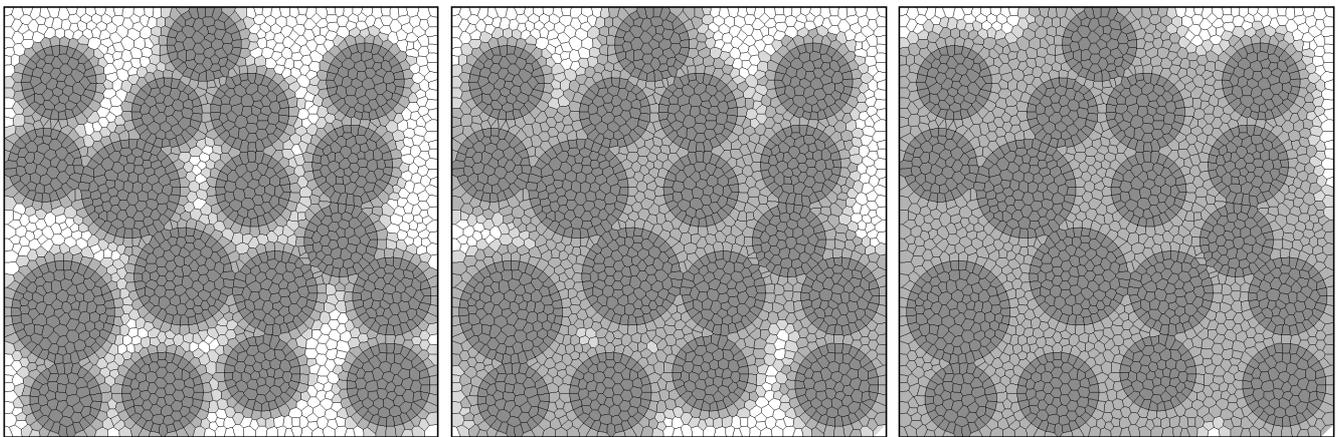
Fig. 5. The kinetics of solidification – 50% fibres fraction
