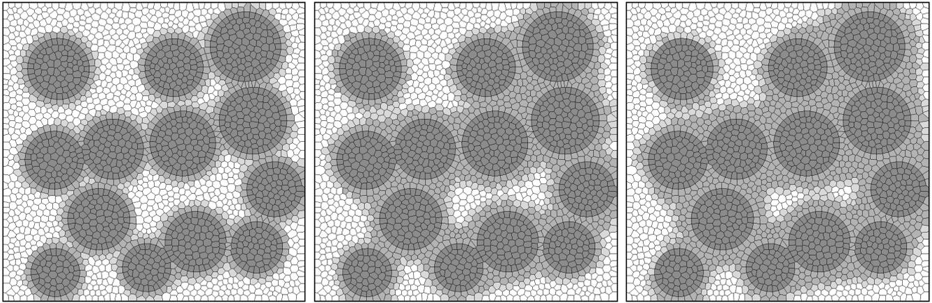
Fig. 4. The kinetics of solidification – 40% fibres fraction
