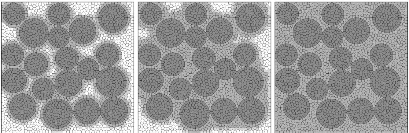
Fig. 6. The kinetics of solidification – 55% fibres fraction
