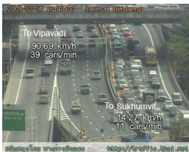
Fig. 7. Image classified as jam traffic by ANN and as light traffic by OR technique.
