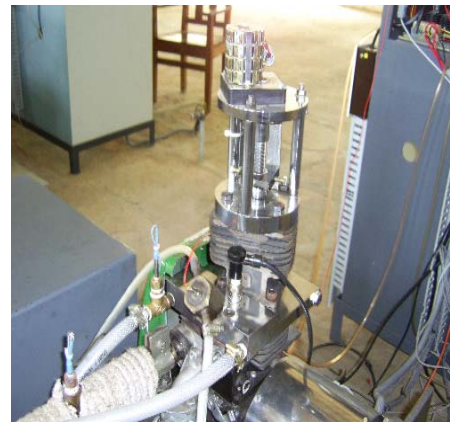
FIG E: 256cc, 3000rpm, Petrol Engine with Movable Head
