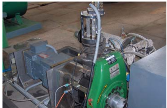
FIG B: 4 S, 256cc, Variable Compression ratio, Variable Spark Advance, Air Cooled Petrol Engine
