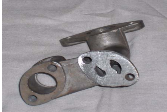
FIG A: Intake Manifold Part with Helical Grooves for Swirl
