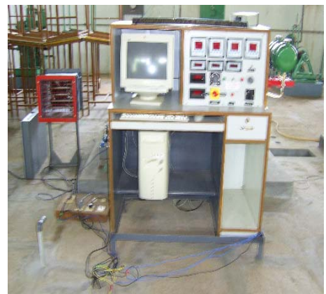
FIG F: Front Control Panel of Fully Computerized Rig
