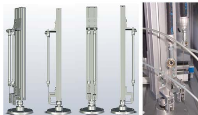
Fig. 7 Construction of the rotation module
