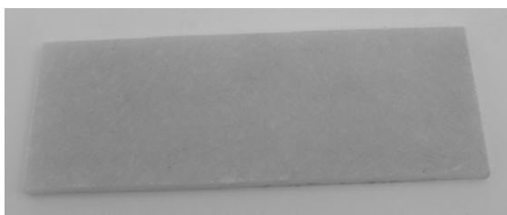
Fig.2 Sample used for impact tests
