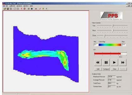
Fig. 6. Screenshot of the software displaying pressure distribution.
