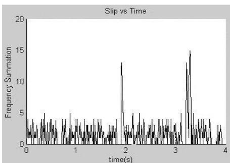
Fig. 12. Frequency summation of the tactile elements for the cork ball experiment.
