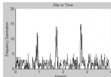
Fig. 10. Frequency summation of the tactile elements for the glass bottle experiment.
