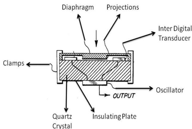
Fig. 1. Internal construction of a tactile array cell.
