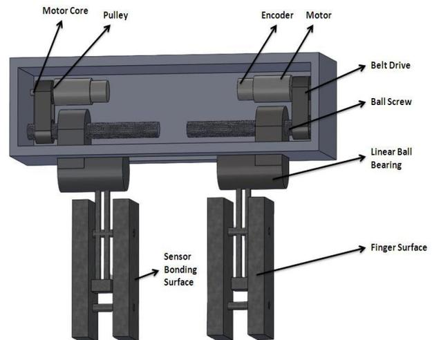
Fig. 4. Cross-sectional view of the gripping system.
