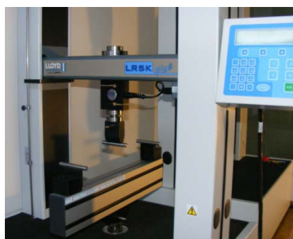
Fig. 3. Bending device (three point method) of the testing machine
