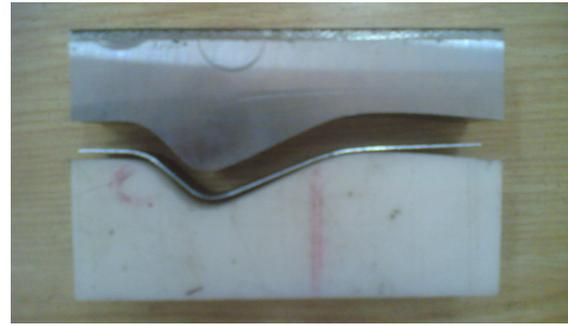
Figure 9. Asymmetric channel forming test.
