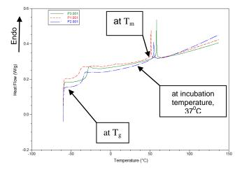
Fig. 5. DSC shows heat flow as a function of temperature for the three compositions of cholesteryl liquid crystals. No exothermic or endothermic activities were observed at 37°C.
