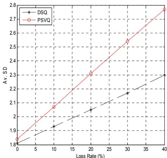
Figure 6. Average LSF spectral distortion for DSQ and PSVQ.
