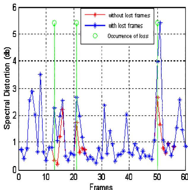
Figure 1. LSF spectral distortion error propagation of G.723.1 coded speech
