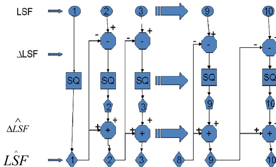
Figure 4 LSF Differential Scalar Quantization
