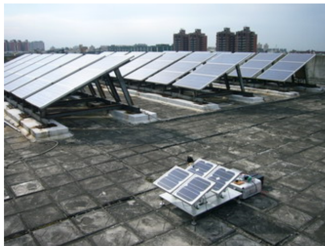
Fig. 9. The picture of proposed solar tracking system placed by a large-scale fixed angle type system.
