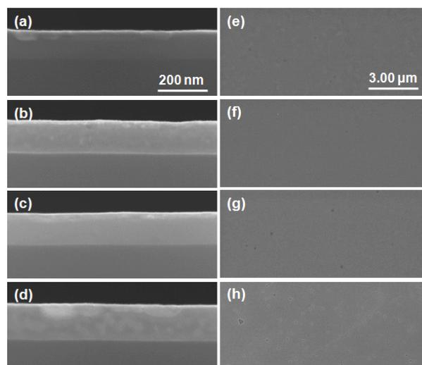
Fig. 7. Cross-sectional (a-d) and plan-view (e-h) FESEM images after post-germanidation annealing with oxide capping layer for un-doped (a, e) at 500°C and B<sub>11</sub>- (b, f) at 575°C, BF<sub>2</sub>- (c, g) at 575°C and As- (d, h) doped substrates at 550°C.
