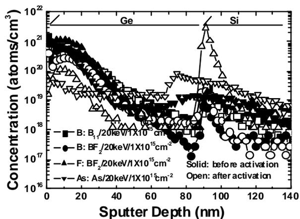
Fig. 1. SIMS depth profile of B<sub>11</sub>, BF<sub>2</sub> and As doped on Ge-on-Si substrate before and after the dopant activation with a RTP at 550 °C for 60 sec.
