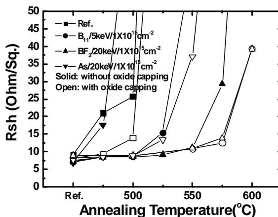
Fig. 3. Sheet resistance of NiGe with and without oxide capping layer on doped Ge-on-Si substrate as a function of post-germanidation annealing temperatures.
