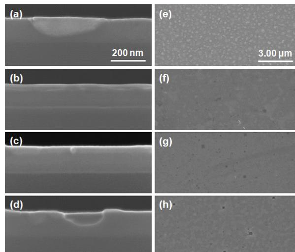
Fig. 6. Cross-sectional (a-d) and plan-view (e-h) FESEM images after post-germanidation annealing without oxide capping layer for un-doped (a, e) at 500°C and B<sub>11</sub>- (b, f) at 525°C, BF<sub>2</sub>- (c, g) at 550°C and As- (d, h) doped substrates at 500°C.
