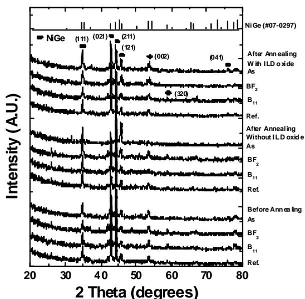
Fig. 4. XRD spectra of Ni germanide with and without oxide capping layer on un-doped, B<sub>11</sub>-, BF<sub>2</sub>-, and As-doped substrates before and after post-germanidation annealing.
