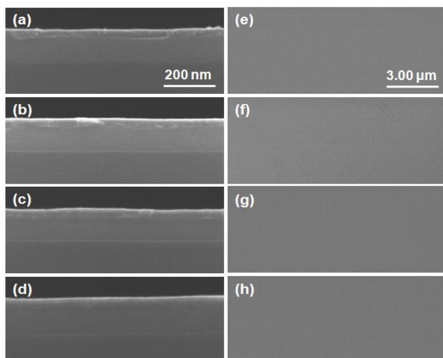
Fig. 5. Cross-sectional (a-d) and plan-view (e-h) FESEM images after germanide formation, i.e., before post-germanidation annealing for un-doped (a, e) and B<sub>11</sub>- (b, f), BF<sub>2</sub>- (c, g) and As- (d, h) doped substrates.
