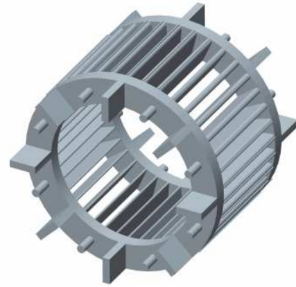
Figure 1. Scheme of a rotor cage of an induction machine
