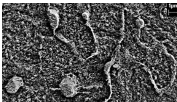
Fig-6: Higher magnified Scanning Electron Microscopy image of 2.1 mm thick layer showing discrete copper channels.
