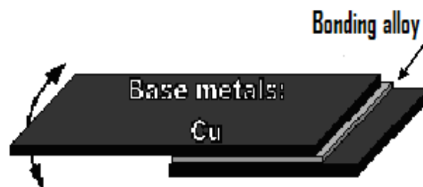
Fig.1. Copper lamellar elements assembling
