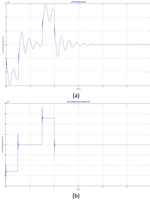
Fig. 11 Displacement of spindle due to input of ball nut
