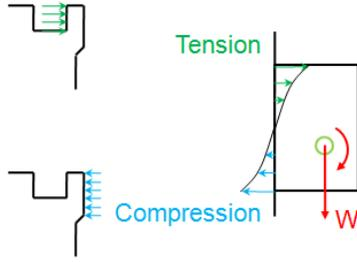
Fig. 2 Different stiffness in vertical sliding guide
