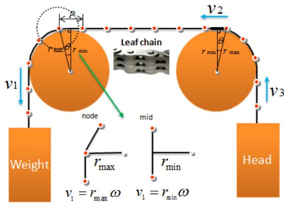
Fig. 12 Velocity difference by chain assembly
