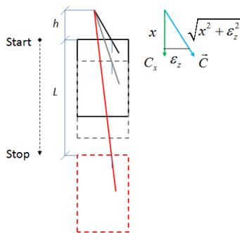
Fig. 6 Misalignment of connecting chain/wire to spindle head
