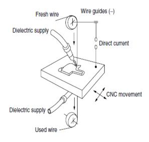
**Fig. 1** – Wire electric discharge machining (WEDM) model [3]
