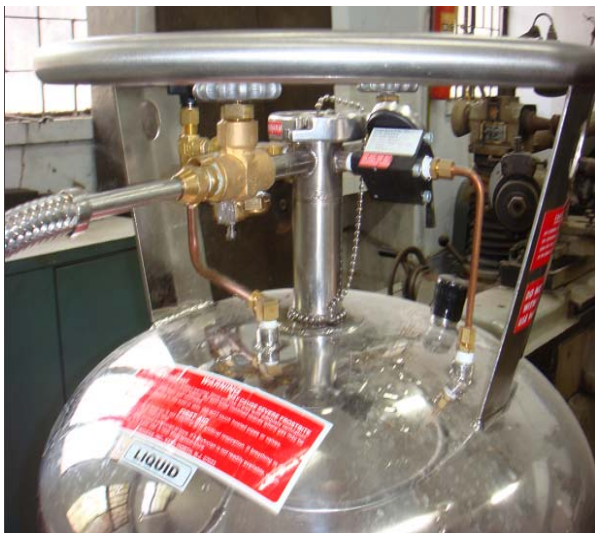
(c) Cryogenic dewar at 4 bar pressure
