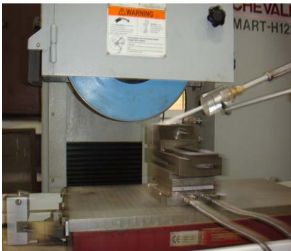
(b) Cryogenic applied on grinding zone
