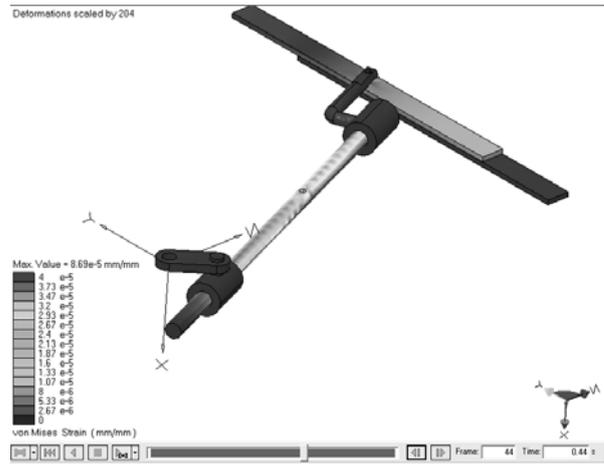
Fig.19.The strain distribution for the mechanism assembly
