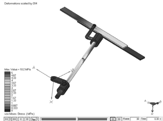
Fig.17.The stress distribution for the mechanism assembly
