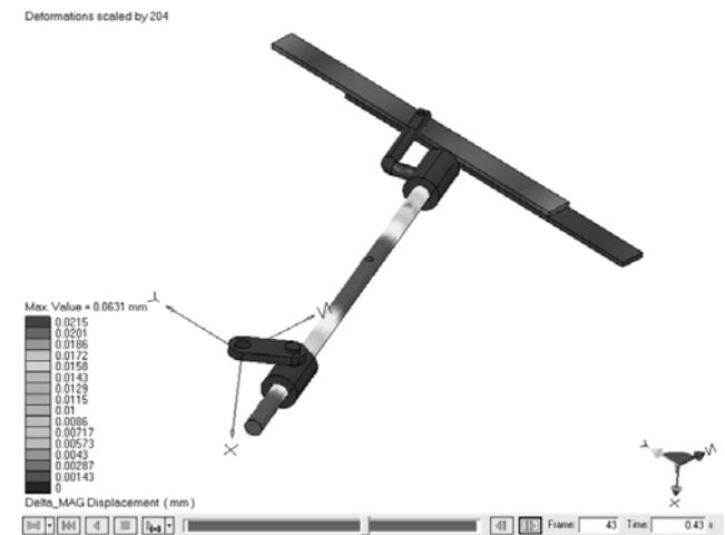
Fig.18.The displacements distribution for the mechanism assembly
