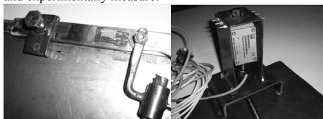
**Fig.15.**Transducers to measure the resistance force and of the motor torque
