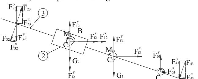
**Fig.6.** The scheme of the forces and moment which act upon the dyad  $B_r B_r C$
