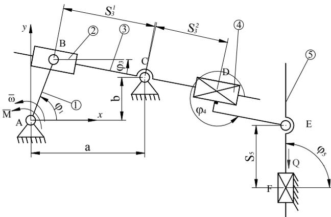
**Fig.4.**The calculus scheme for the mechanism kinematic model
