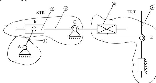
Fig.3. The structural decompose in Assur groups
