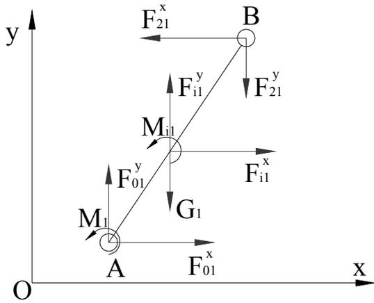
Fig.7. The scheme of the forces and moments that acts upon the motor element
