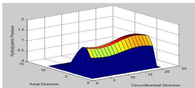
Fig: 10 Hydrodynamic Pressure Field at 640° Crank Angle
