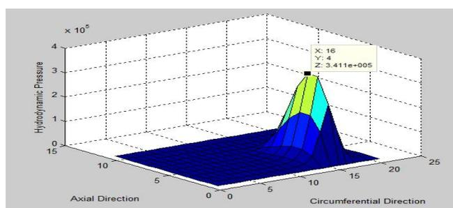
Fig: 7 Hydrodynamic Pressure Field at 370° Crank Angle
