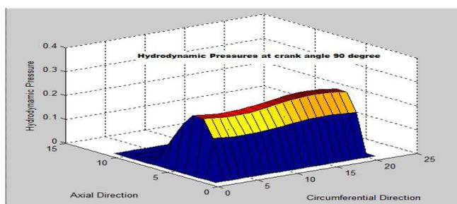
Fig:5 Hydrodynamic Pressure Field at 90° Crank Angle
