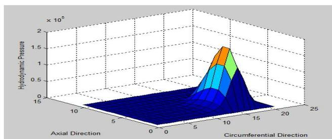
Fig: 8 Hydrodynamic Pressure Field at 400° Crank Angle
