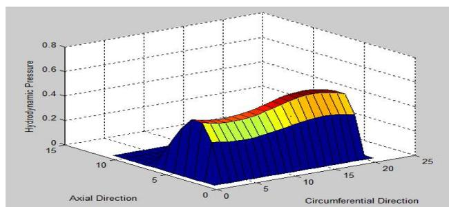
Fig:6 Hydrodynamic Pressure Field at 200° Crank Angle
