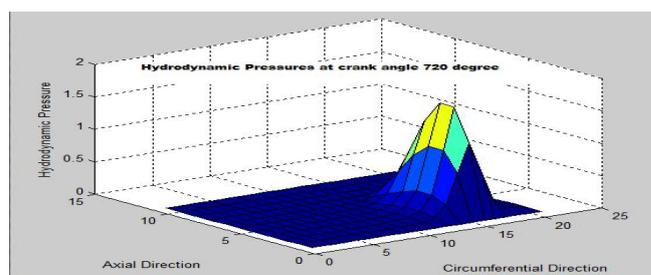
Fig: 12 Hydrodynamic Pressure Field at 720° Crank Angle
