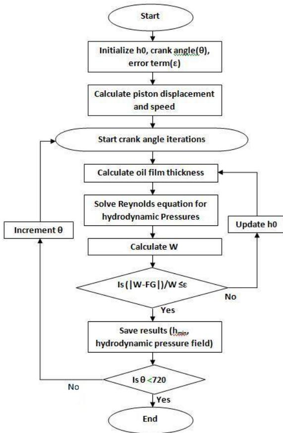
Fig:2 Flowchart of Computational Scheme
