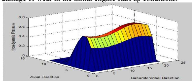
Fig: 11 Hydrodynamic Pressure Field at 690° Crank Angle
