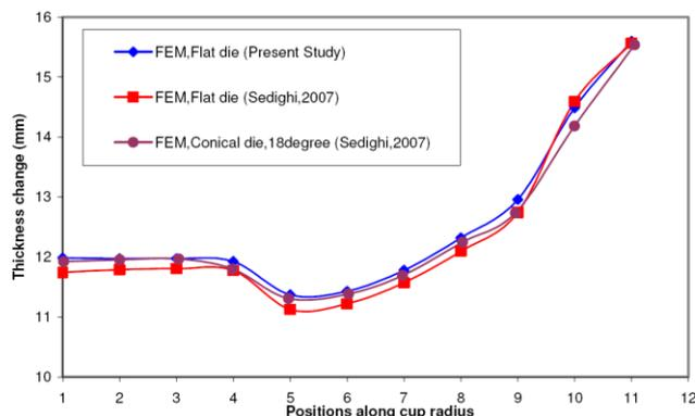
Fig10. Simulation result of changing blank thickness at the end of cold deep drawing
