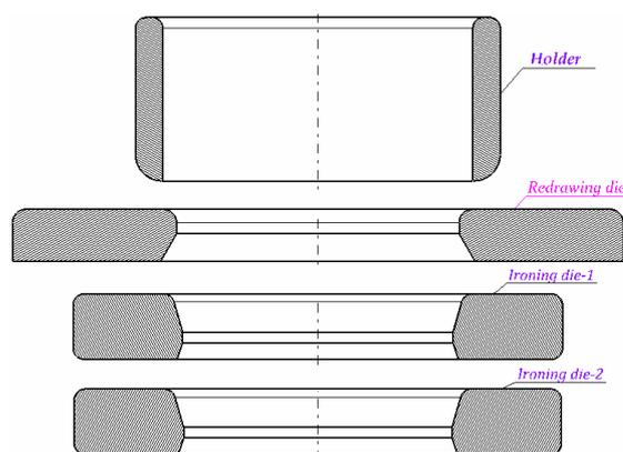
Fig11. schematic model of the redrawing and ironing dies
