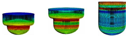
Fig13. Cold redrawing stages of CNG
