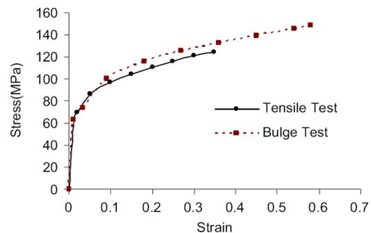
Fig7. Stress-strain curves resulted from tensile test and bulge test [6]
