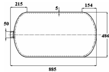
Fig5. Geometrical properties of the CNG vessel [6]
