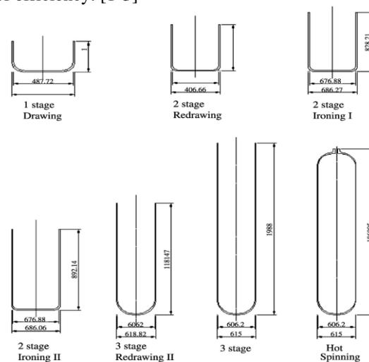
Fig1. Primary stages of the steel core forming a CNG vessel [2]
