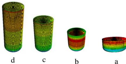
Fig4. Manufacturing stages: a) cold deep drawing b) cold redrawing c) first ironing d) second ironing [6]
