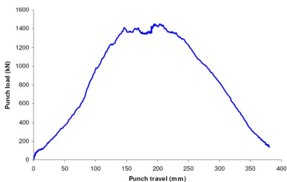
Fig9. Force-displacement curve of the punch in drawing stage (drawing ratio 1.7)
