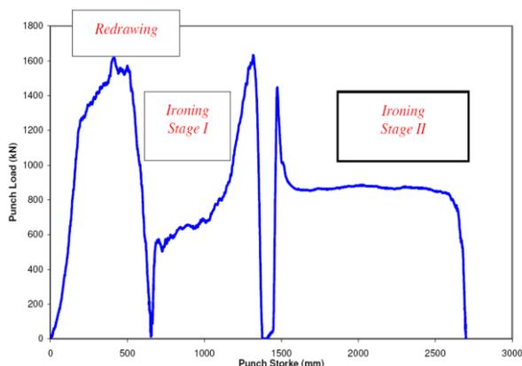
Fig16. Force-displacement curve in redrawing an ironing of the first and second stages
