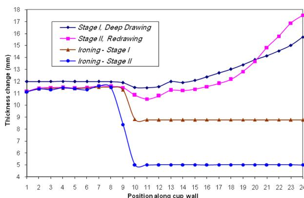
Fig18. Comparison of wall thickness in different stage of forming
