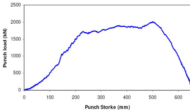
Fig12. Force-displacement curve of the punch in cold redrawing
