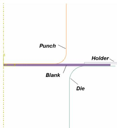
Fig8. Axisymmetric model for simulation of cold deep drawing
