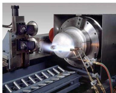
Fig2. Heat rotational forming (spinning) of the CNG dome [1]
