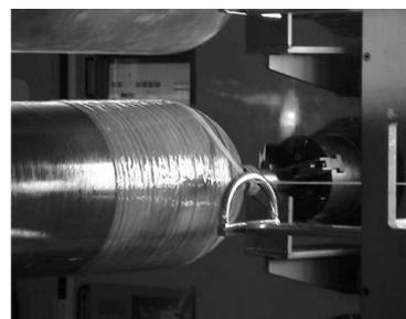
Fig3. Wrapping composite priming around the CNG vessel resin [1]
