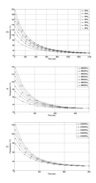
**Fig. 2** Cooling curves, variation of the specimen's temperature with time for different initial input power and three selected pressure: a)18Pa, b)88500Pa, c)220000Pa.
